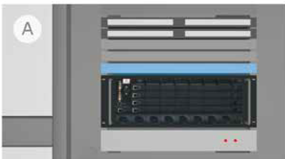
System expansion with IT and telecommunication value-added services in 19" cabinet consisting of servers, system switches for using existing 2-wire installations.t
