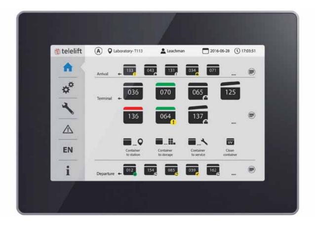
Operation of the Telelift system is easy and self-explanatory. The new terminal has 6 main entry areas for users: home, settings, service, error messages, language setting and operating manual:
