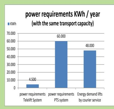
The energy requirement of a Telelift system represents one tenth of the energy requirements of a pneumatic tube system. The message service performed by pneumatic tube systems additionally requires 10 times the energy of an alternative Telelift system.
